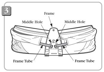
• Position the ends of the frame tubes against the middle holes in a frame.
